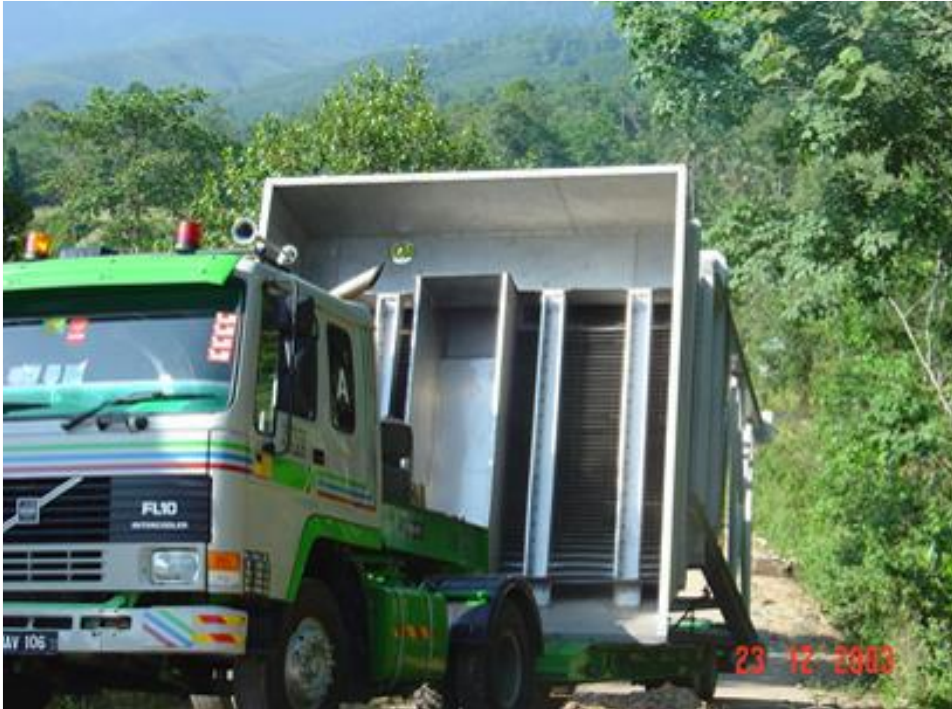
Lamella settler being transported along forest track
