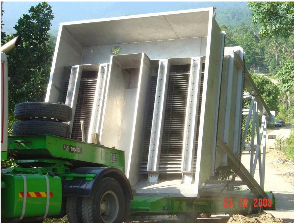
Lamella settler being transported along forest track
