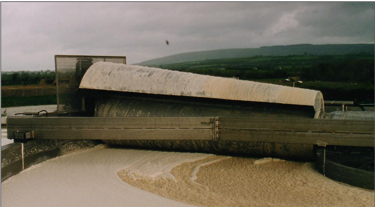
View of SPC showing removal of floated fats, oils & greases with spiral scoop.
